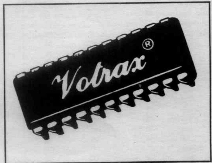
Figure 1. Votrax ® SC-01 Speech Synthesizer
